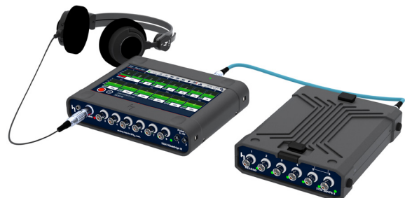
labVF6 II HEADlab module connected to the HEADlink+ interface of SQuadriga III via HEADlink
