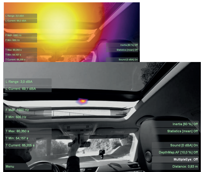
The same measurement situation without Neural Deconvolution (smaller picture above) and with Neural Deconvolution.
