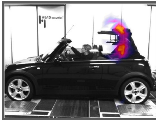
Figure 8: Sound source localization by means of beamforming
