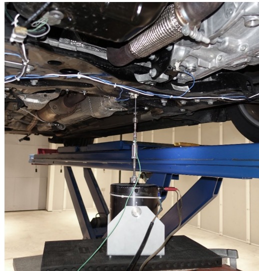
Coupling of a shaker with stinger
